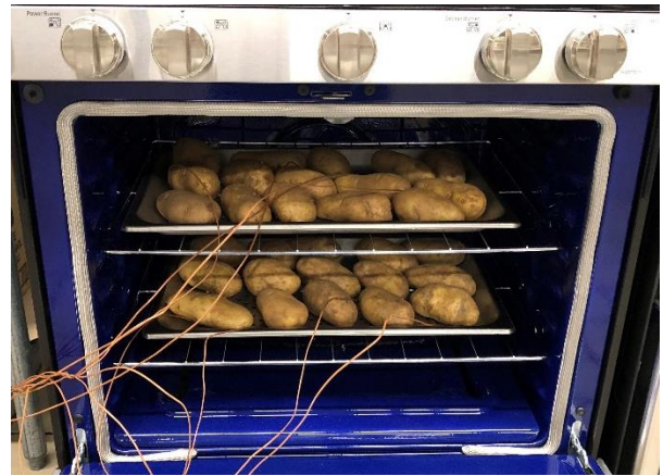
Figure 3: ASTM Cook Test with Russet Potatoes
