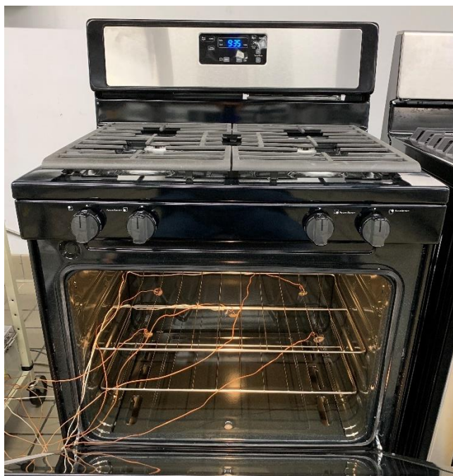
Figure 1: Temperature Calibration and Thermocouple Placement
