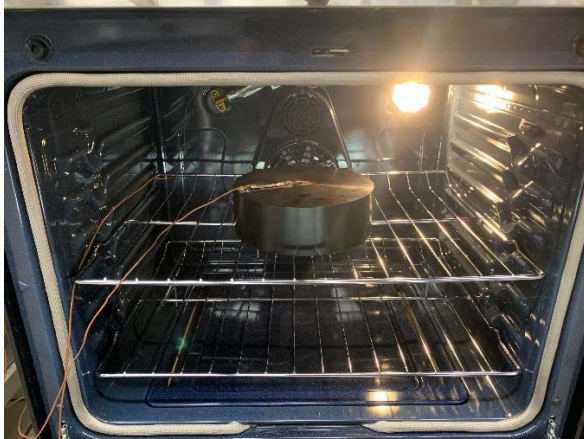
Figure 2: DOE Cook Test with Aluminum Block
